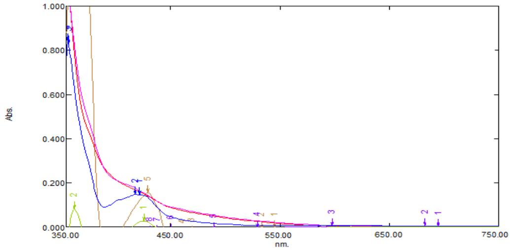
**Fig. 2: UV-Vis spectrum of synthesized silver nanoparticles showing absorbance peak at 420.00 nm to 440.00 nm.**
